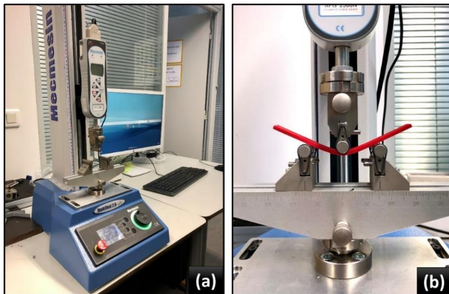
Figure 63 – (a) Bending Test Machine in LPDS; (b) Bending test on a flexural sample.
