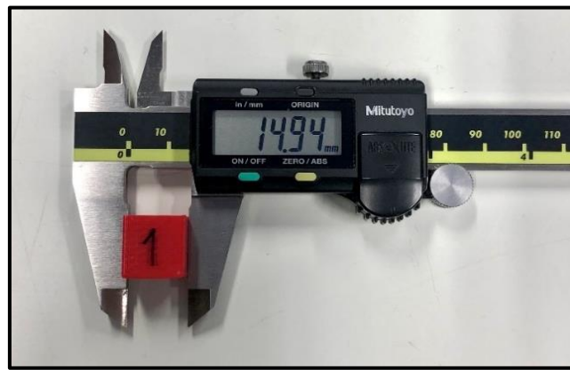
Figure 51 - Test cube being measured with a Mitutoyo TM caliper.
