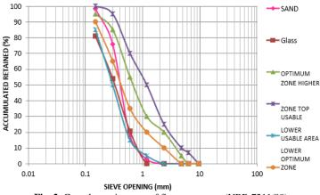
Fig. 2. Granulometric curve of fine aggregates (NBR 7211/09).
