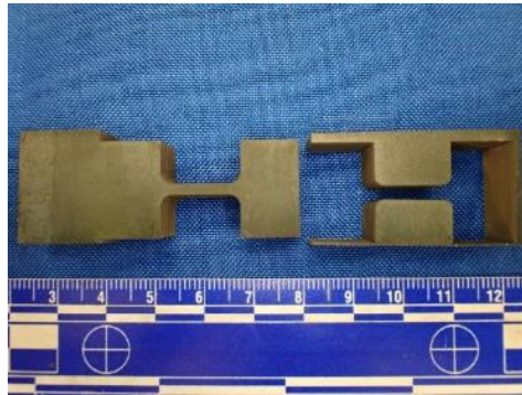
Figure 5-4: Meso samples directly after the wire EDM process
