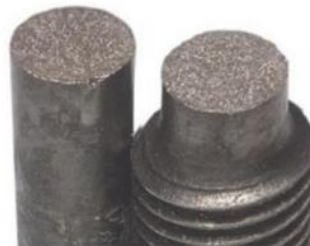
Figure 6-7: Fracture surfaces of a brittle fracture. Note the flat fracture surface (modified from [132])
