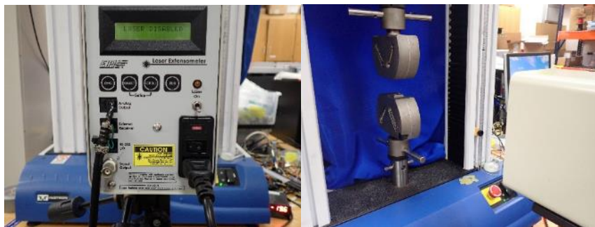
Figure 5-6: Non-contact laser extensometer and Instron 3369 Dual Column Tabletop Testing System
