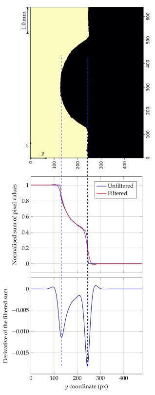
**Figure 6.** Operations associated with detecting the coordinate of the substrate's interface with the background, for line bead 1 (the first derivative's global minimum is one potential indicator of the substrate's starting location).
