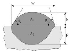
Figure 1. Schematic representation of DED-produced line bead properties.
