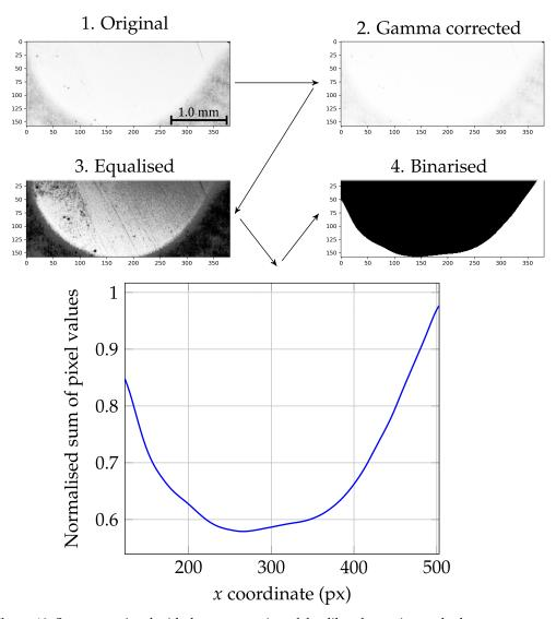
**Figure 10.** Stages associated with the segmentation of the diluted zone (example shown corresponds to track 1).
