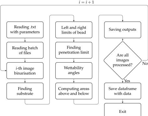
Figure 3. Developed algorithm's flowchart: user inputs limited to first step.
