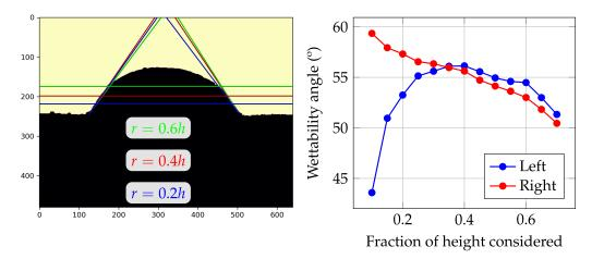
**Figure 9.** Influence of the height *r* considered when computing wettability angles (example shown pertains to track 1).
