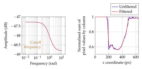
**Figure 5.** Frequency response pertaining to the sum of pixel values, by column, of the image belonging to track 33.
