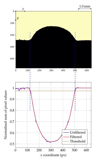
**Figure 7.** The detection of the bead's limits through the interception of the normalised sum of pixel values with an established threshold (shown track equates to track 1).
