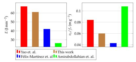
**Figure 13.** Comparison between the specific energy *E* and ratio between scanning speed and feeding rate  $v_s/f_r$  between the present work and other research: Yao et al. [29], Félix-Marínez et al. [28] and Amirabdollahian et al. [39]. The parameters shown by [28] were optimised for dilution  $\geq$  10%, and the work by Yao et al. [29] where the parameters resulted in a specimen with the largest tensile strength.
