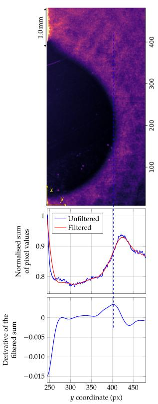
obtaining the dilution proportion, according to Equation (2). Figure 10 illustrates the several steps before the binarised dilution zone is obtained.
