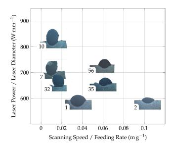
**Figure 11.** Parametrisation window overlayed with cross-section images of the produced beads: Lower ratios between the scanning speed and feeding rate lead to low dilution proportions and large wettability angles, while increased ratios lead to decreased bead heights.
