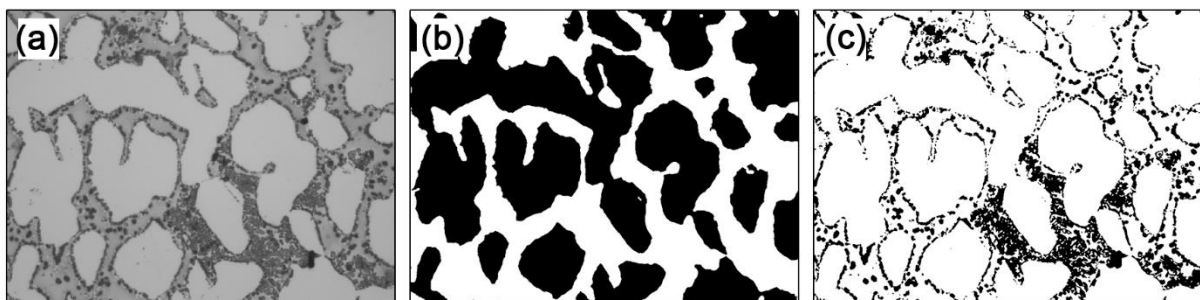
Figure 9 – Segmentation of optical micrographs using a thresholding-based histogram algorithm; a) Optical micrograph showing brighter \gamma -phase, middle-grey \delta -phase and dark precipitates of secondary phases; b) binary image where black areas correspond to \gamma -phase; c) binary image where black areas correspond to precipitates of secondary phases.
