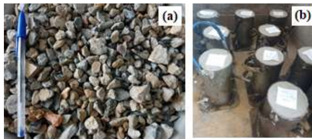
Figure 1: (a) Coarse aggregate after treatment and (b) modeled specimen
