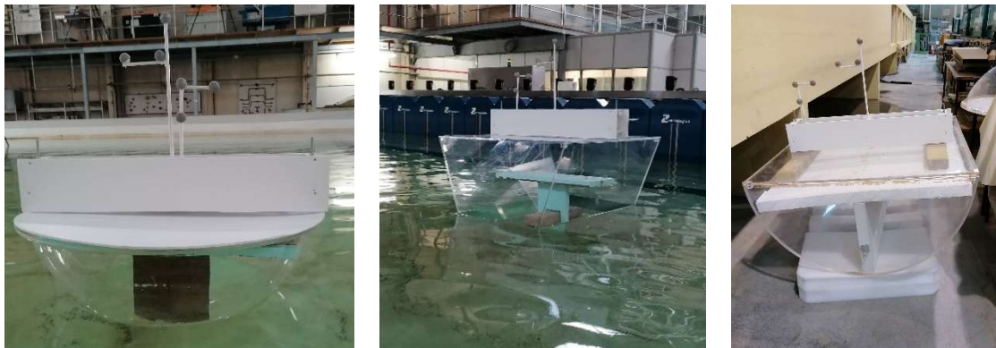
Figure 24: E-Motions physical models: half-sphere, trapezoidal prism and half-cylinder (from left to right).
