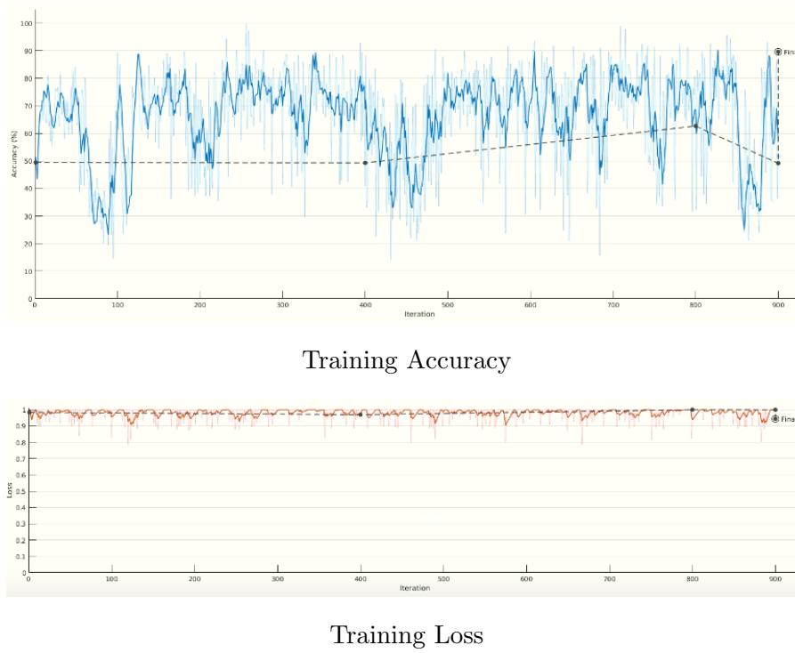
Figure 5.9: Accuracy and loss on the network training the data set with the HU mask. The blue line represents train accuracy, the red line represents train loss and the black lines are validation accuracy (first image) and validation loss (second image)
