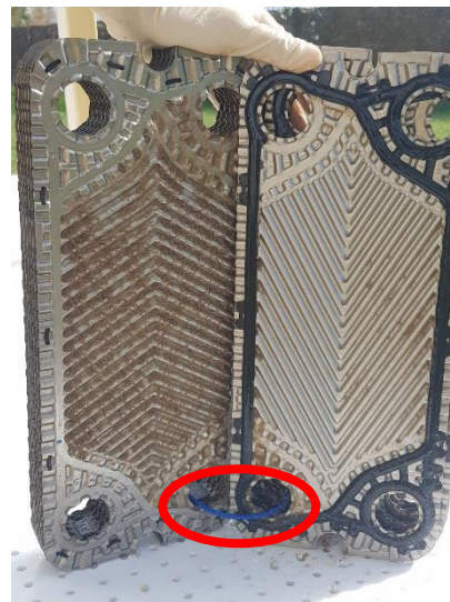
Figure 2 - Inner plates dirty and clean
