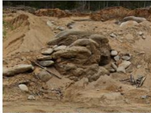
Figure 7: Picture of the quarry at Tranøy shows sandy to grussy type material. Core stones indicate potential bedrock weathering, which is common in this area and possibly even in-situ .
