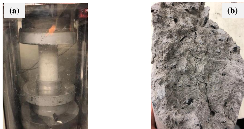
Figure 7 (a) Compression test and (b) Surface of the BM5 after compression test
