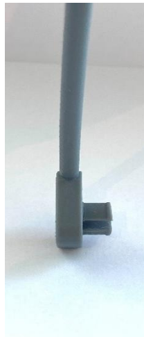
Figure 97- Rod joint prototype front view
