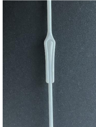
Figure 58- Zoom of snap fit joint of the rod
