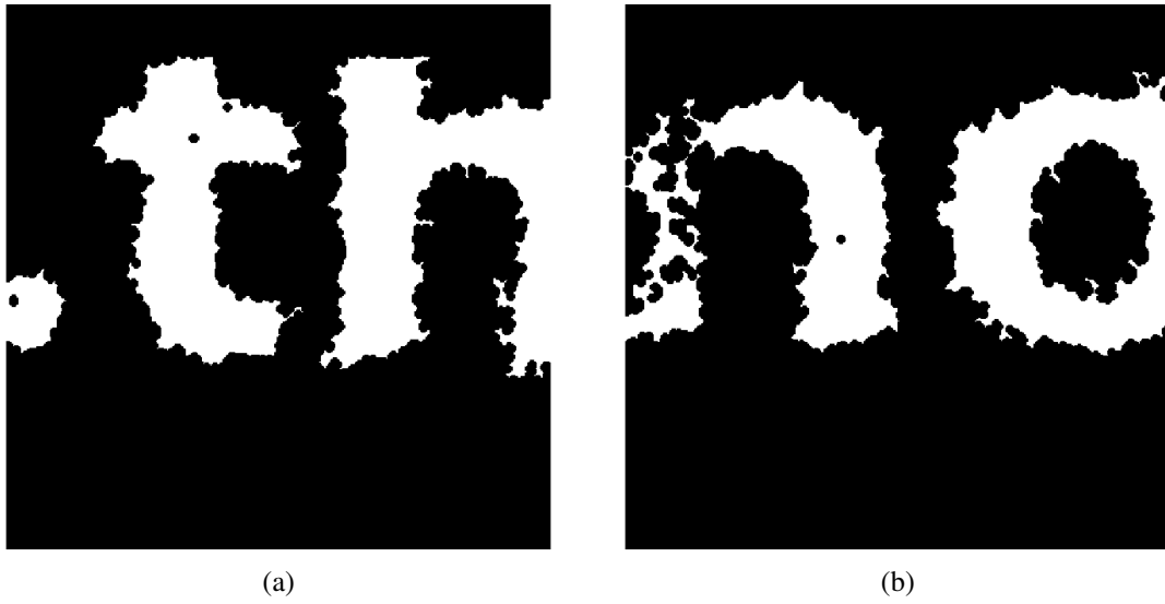
Figure 6.11: En face images of the volume acquired at 0^\circ a) and 5^\circ b) after area opening
