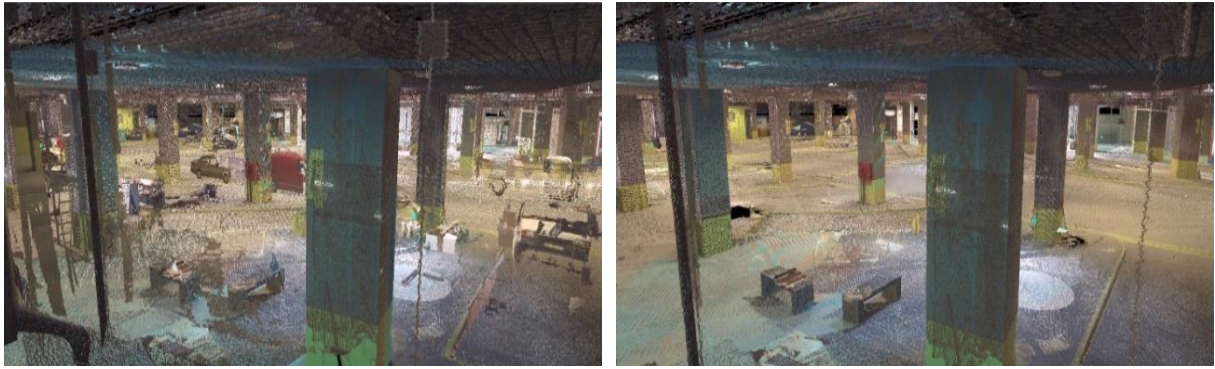
Figure 3.14 – Example of a point cloud before (left) and after (right) completing the cleaning task
