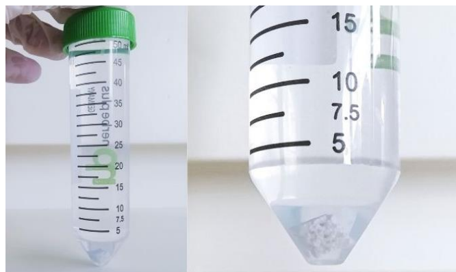
Figure 6. Representative image of the scaffolds position during immersion in simulated body fluid (SBF), showing that the scaffold surface had minimal contact with the falcon tube.
