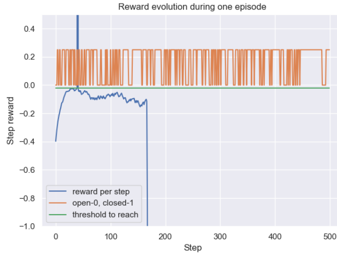
(a) Reward Function 2 and Episode 154. The reward function suggests that the cube was projected at step 90 and flies away until step 140. This collision was so dramatic that the object reentered the environment from then on, and the gripper remains to explore the workspace without the possibility to change that.
