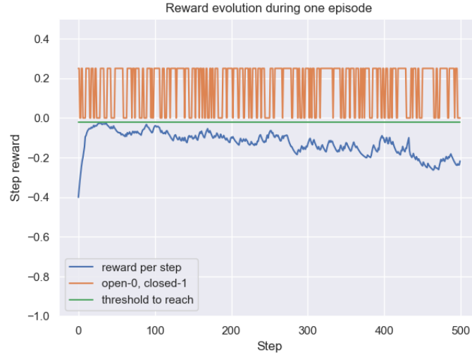
(a) Reward Function 1 and Episode 4. The reward function and the coordinates' log suggest that the cube exited the action space at step 271, ending the episode at X_{object} = (0.58185959; 0.15100859; 0.02397567] . The gripper starts approaching the object and gets close to it around step 30 as the reward line approaches the threshold line. This episode does not receive rewards as lower as the previous (Fig. B.2a) because it ends closer to the action space's limits.
