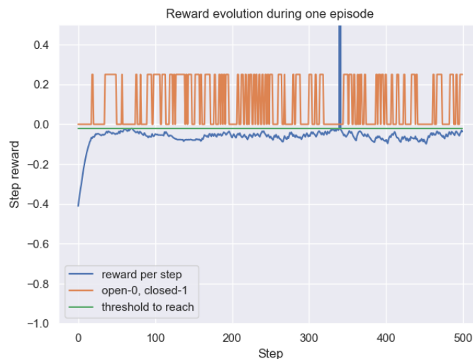
(a) Reward Function 5 and Episode 609. The reward function suggests the agent approached the object and moved away several times during the episode. The agent only performed the reaching at step 340. then the agent moved past the point and failed to pick the object before the episode reached 500 steps.
