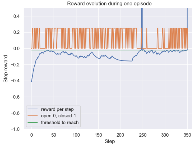
(a) Reward Function 1 and Episode 370. The agent reaching the object at step 248 and picking the object at step 351. The agent moves the gripper near the object at an early stage but is not successful. This episode demonstrates where the agent is not optimised, and there are around 100 steps of slack between reaching and picking. The main reason for the episode to last longer might be related to the alternation between gripper's fingers states, moving the cube to different positions
