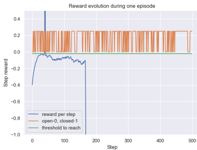
(a) Reward Function 2 and Episode 165. The reward function suggests that the cube was reached around step 30. Then, the gripper moved past the object centre and collided with it, around step 170. The following rewards were -11.25 , which ended up penalising the good cube approach.
