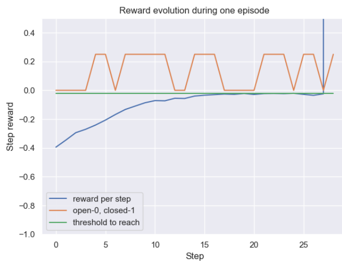
(a) Reward Function 1 and Episode 64. The agent succeeds in reaching and picking the object simultaneously. This behaviour is optimised when compared to the expert behaviour that performs those in consecutive steps
