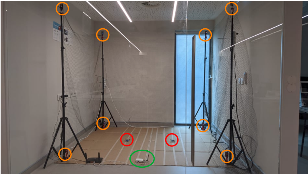
Figure 3.8: Test arena at Capgemini Engineering. Color code: Orange - LPS anchors (bottom right one is used as the referencial for the odom frame), Red - MAVs, Green - Ground Station (Raspberry Pi) with a crazyradio PA
