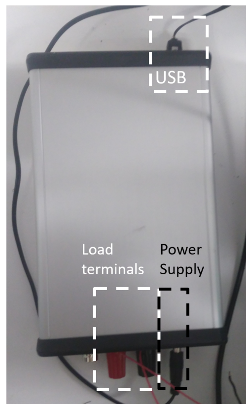
Figure 14: Box of Resistances with built-in Arduino, labeled.
