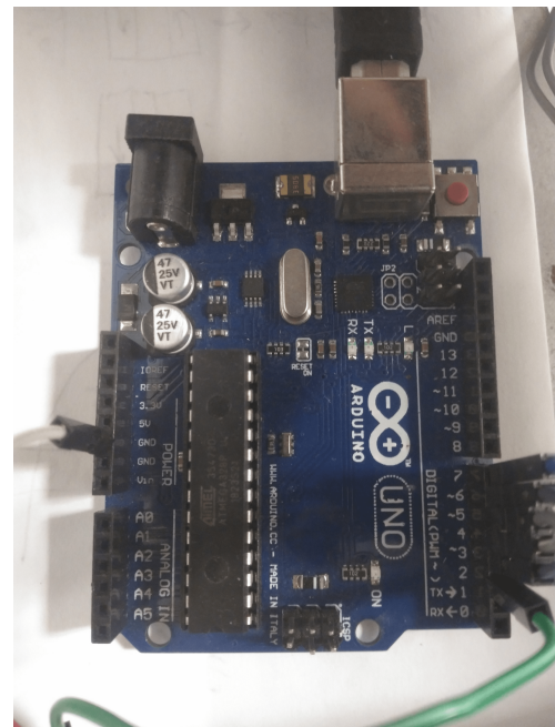
Figure 11: Picture of Arduino 1, where the digital pins are on the bottom right corner. Notice the reset button on the top right corner in red.
