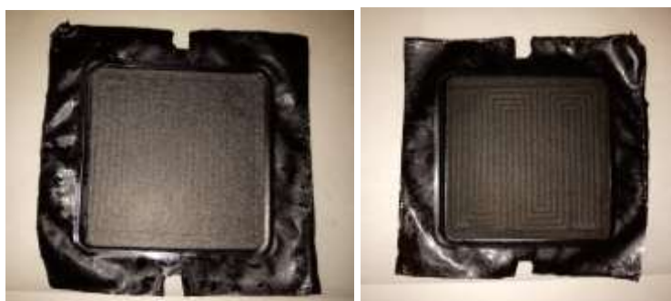
Figure 3.14 - Burnt electrode at the end of the stability test for the PBI membrane with 2% GO.
