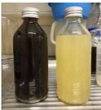
Figure 3.5 - OMW sample before (left) and after (right) AO treatment at 200 mA/cm 2 .
