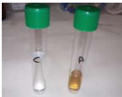
Figure A.6.1 - Samples for stability test for PBI membrane with 2% GO from cathode (C) and anode (A) purge.
