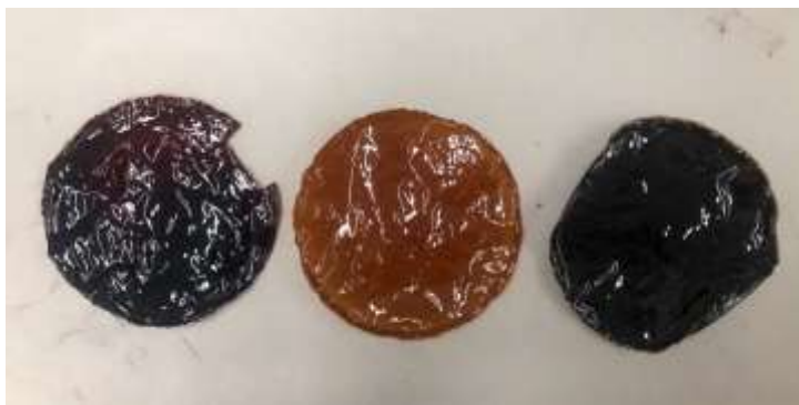
Figure 3.7 - Thermally cured standard PBI membrane, standard PBI membrane, and PBI membrane with 2% GO (from left to right).
