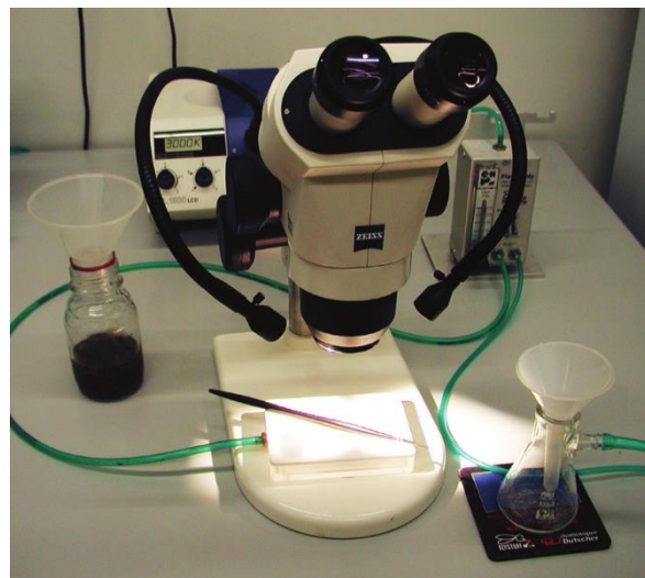
Figure 10 - Typical workbench when dealing with Drosophila m. . A magnifying glass or stereomicroscope, a carbon dioxide pad, a fly morgue containing ethanol, a brush and a light source. Adapted from [166].
