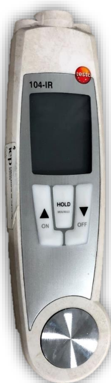
Figure 4. Infrared thermometer used for temperature control - Testo 104-IR .
