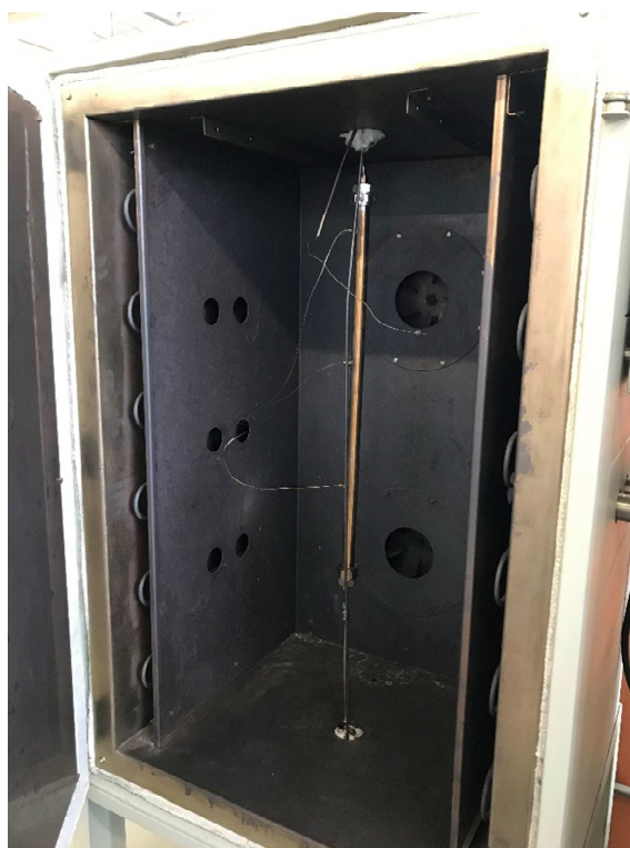
Figure 3.8: Fixed Bed Column packed with MIL-100(Fe) inside the oven with three internal and one external thermocouples.
