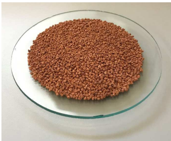
Figure 3.4: MIL-100(Fe) granular sample used in the fixed bed and gravimetric experiments
