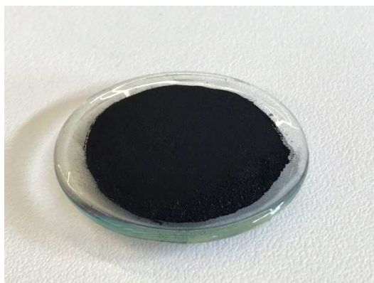
Figure 3.1: Maxsorb powdered sample used in the adsorption equilibrium gravimetric experiments
