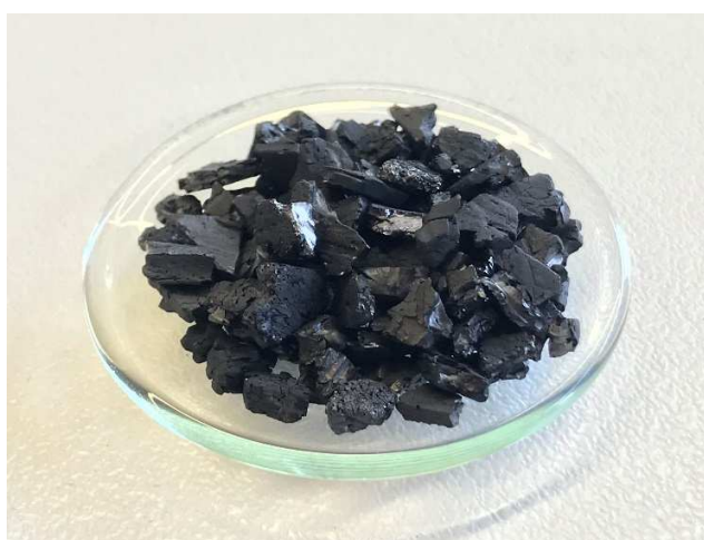
Figure 3.2: CarboTech DGK granules sample used in the adsorption equilibrium gravimetric experiments
