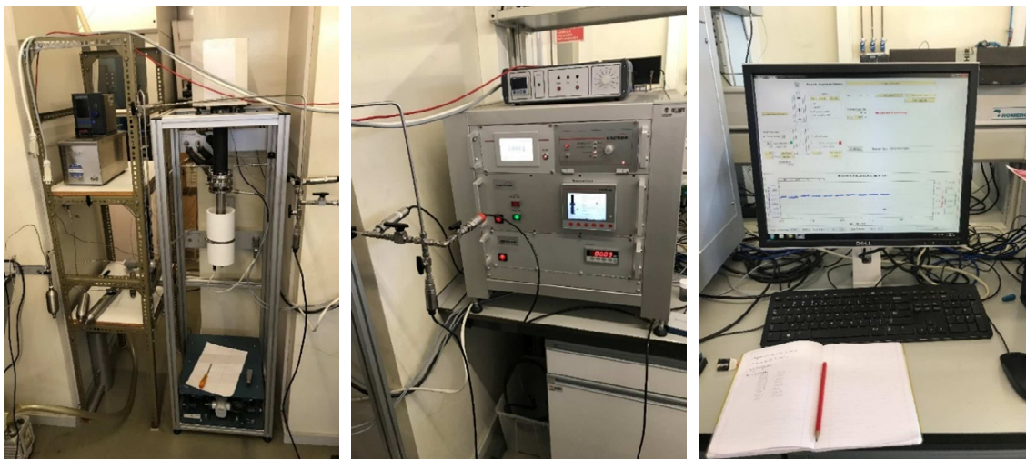
Figure 3.5: Magnetic Suspension balance Rubotherm (a), Electronic Control Unit (b) and Data acquisition system (c)
