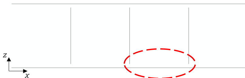
Figure 5.11 – Cohesive elements location in the stiffeners-panels interface mimicking the adhesive’s behaviour.
