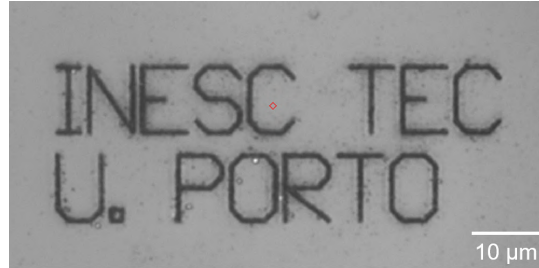
Figure 3.2: Ablation marks formed at the surface of fused silica.
