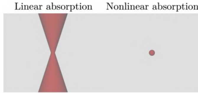
Figure 2.4: Comparison of the modified volume through linear and non-linear absorption. Image was taken from [88].
