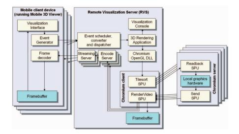
Figure 3.4: Fabrizio Lamberti et al. layout of the proposed three-tier architecture
