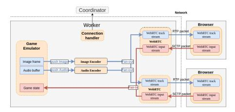
Figure 3.3: Worker internal for CloudRetro
