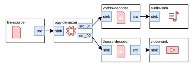
Figure 4.6: GStreamer Pipeline for a basic Ogg player
