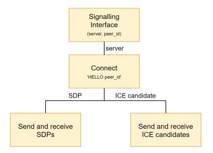
Figure 4.10: Client Signalling Interface
