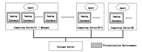
Figure 3.6: Zhang et al. user-level virtualization system architecture
