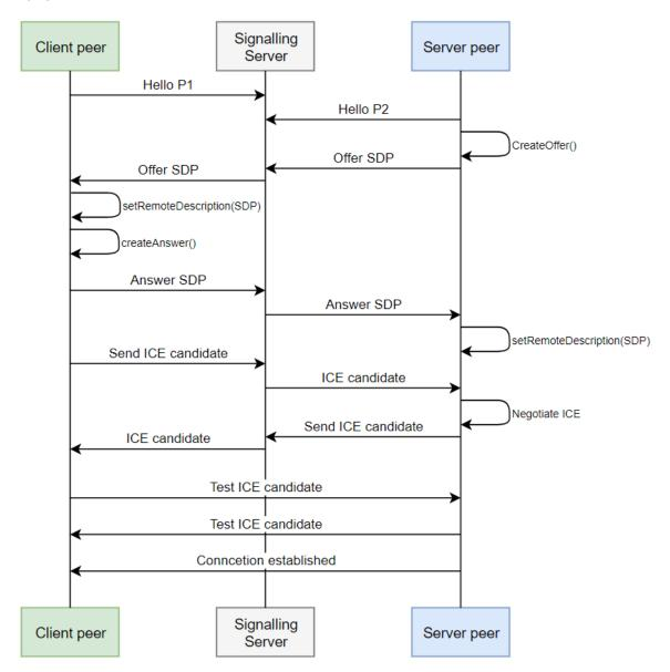
Figure 4.4: Signalling Server Connection Handshake
