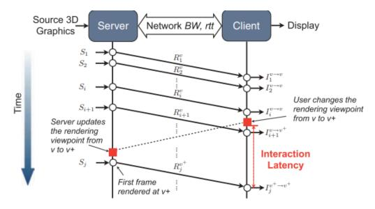
Figure 3.8: Shi et al. remote rendering system framework and an illustration of interaction latency
