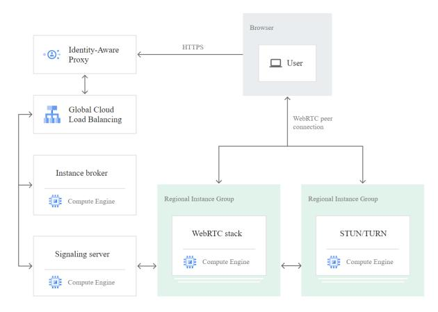
Figure 3.9: GPU-accelerated streaming using WebRTC Architecture
