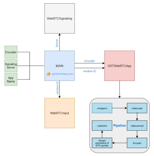
Figure 4.5: GStreamer WebRTC Application Architecture
