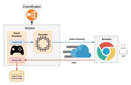
Figure 3.2: High level overview of the system architecture of CloudRetro
