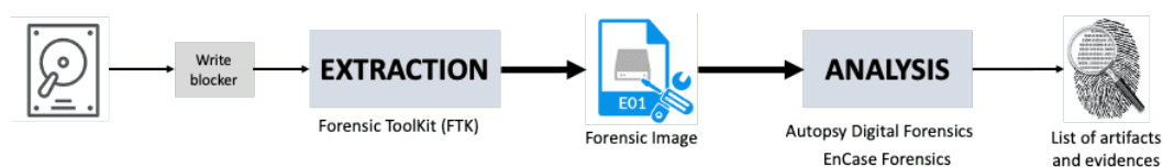
Figure 3.1: Overall procedure to extract and analyze electronic devices.
