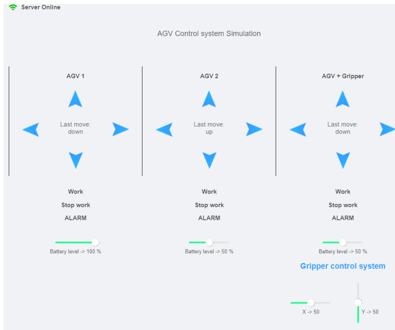
Figure 4.13: AGV Control Software
