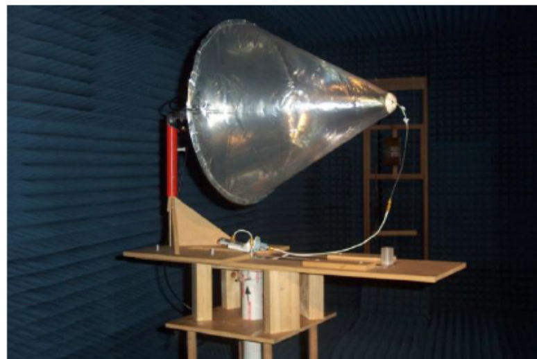
Figure 2.4: Mathers' inflatable antenna under RF measurements, [5]
