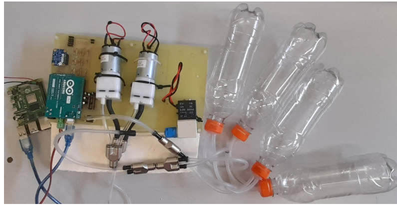
Figure 5.2: Vacuum chamber test pressure control system set up
