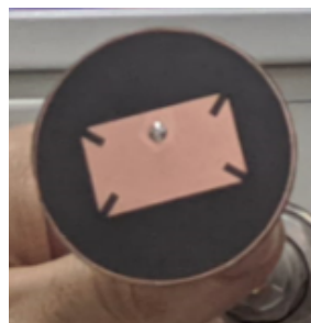
(a) Patch antenna made from dielectric material
