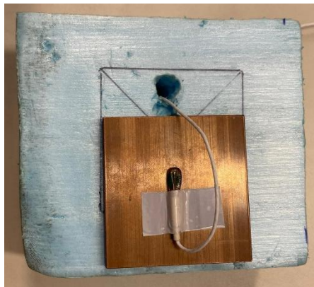
Figure F.1 - Copper sample with the data logger on the extruded polystyrene support.
