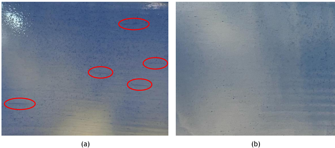
Figure D.1 - Evaluation of formulation dispersion: (a) incomplete dispersion and (b) complete dispersion.
