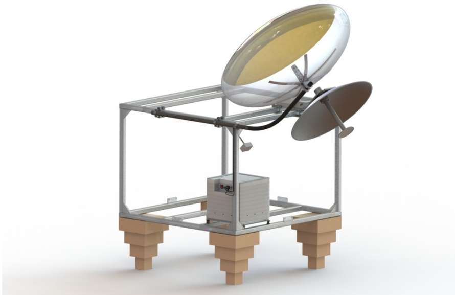
Figure 3.1: BEXUS gondola with the SARIA experiment mounted.
