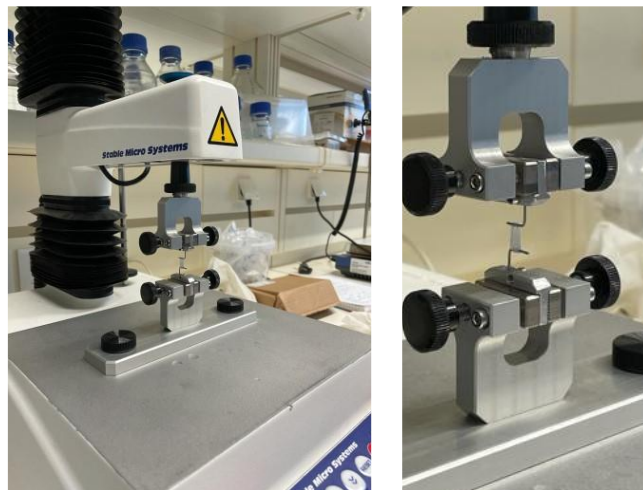
Figure 13 - Texturometer with the customized adapter during a tensile test.
