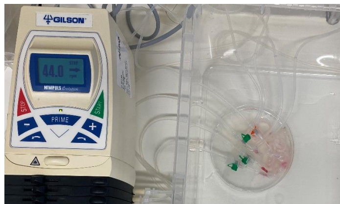
Figure 10 - Automatic decellularization set-up.
