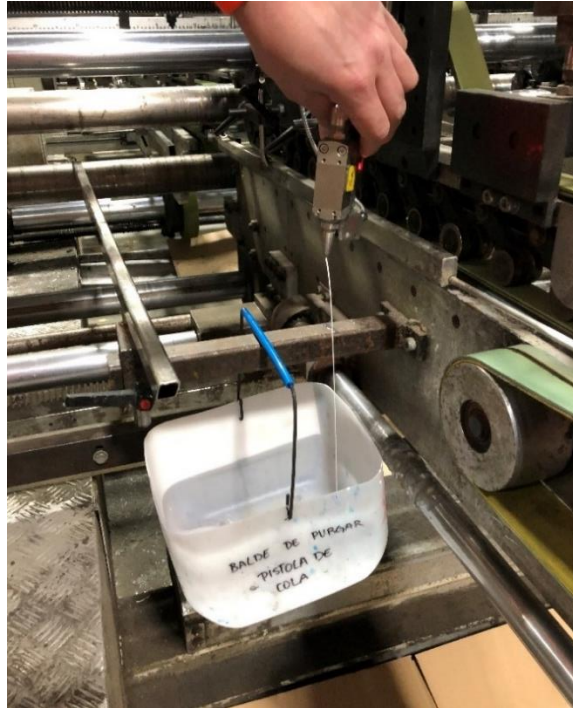
Figura 35 - Balde de purgar as pistolas de cola
