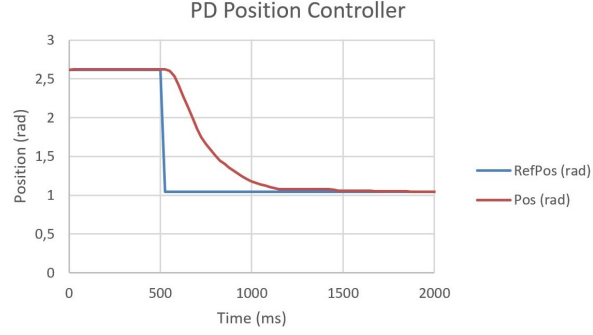
Fig. 9. PD Position Controller response to reference.
