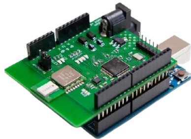
Figure 3.10: Connection between Pozyx tag and Arduino UNO [14]
