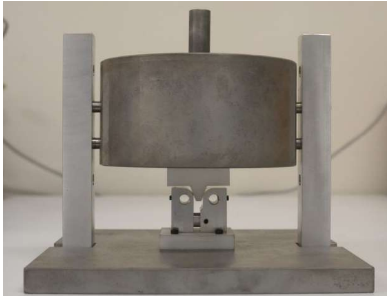
Figure 3.13: Final assembly of the Heating System.
