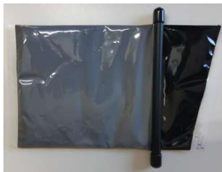
Figure 5.7: ER2220 ® : epoxy resin (silver) and hardener (black).
