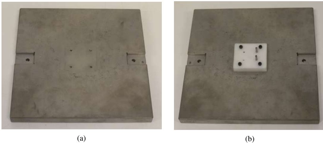
Figure 3.9: Step 1 and 2: placing the table (a) and polymer support plate(b).
