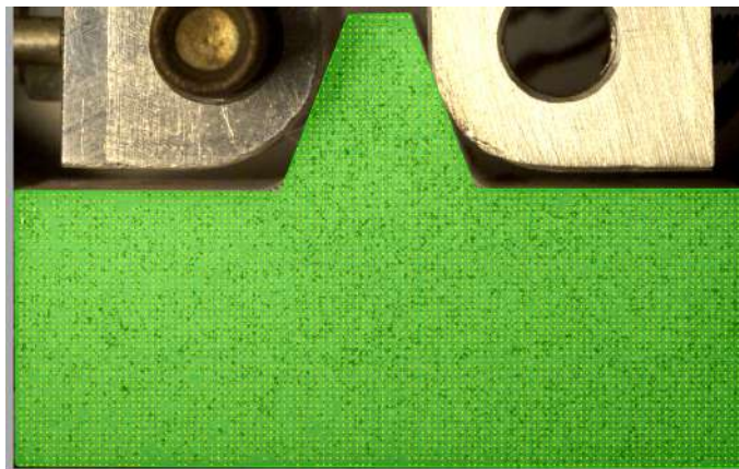
Figure 5.19: Digital Image Correlation Engine (DICE): region of interest and matrix.
