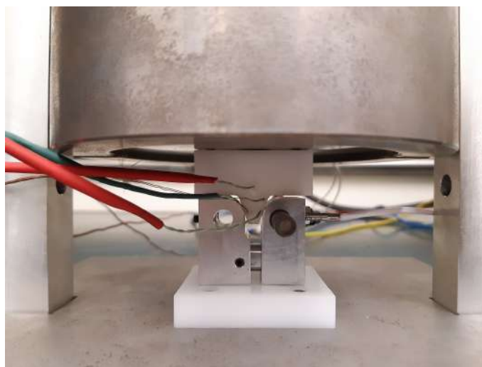
Figure 5.11: Heating System setup with a standard tooth with thermocouple.
