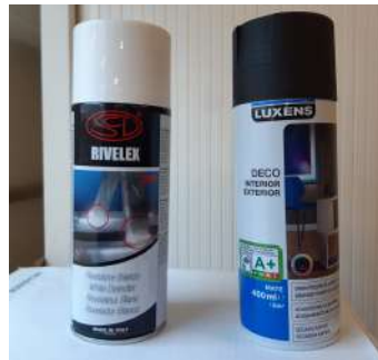
Figure 5.16: Spray used for the speckle pattern: (a) RIVELEX 200 and (b) LUXENS matt black.
