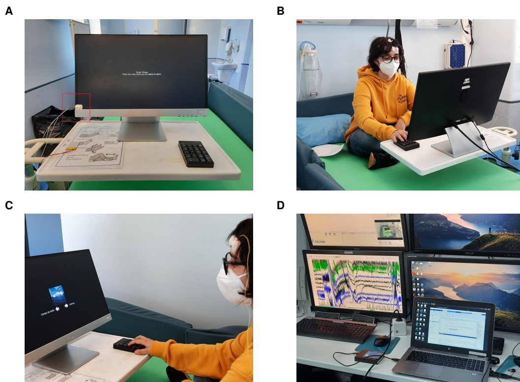
Figure 6.4: Photographs of the in clinic experimental set up. (A) The external display, set on top of an overbed table, and the photoresistor sensor, attached to the bottom-left corner of the screen. (B) Photograph of the participant sitting on one of the EMU's beds at approximately 60 cm from an external monitor. (C) Photograph of the participant using the wireless keypad to convey their responses. (D) Photograph of the monitoring room, including the laptop used to run the routine and the monitoring screens. An intercom is placed in the leftmost corner of the room.
