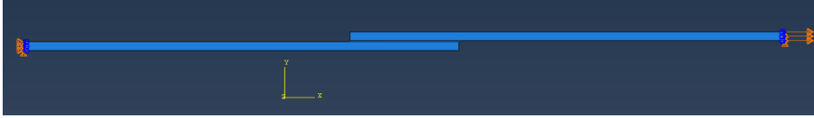
Figure 20: Boundary conditions established for the simulation of the SLJ behavior.
