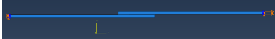
Figure 5: Boundary conditions established for the simulation of the SLJ behavior.
