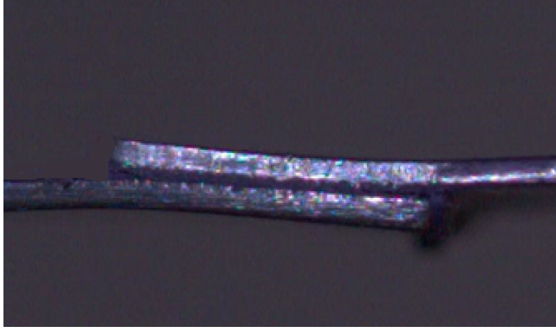
Figure 19: Representative image of the plastic deformation to which the mild steel substrates are subjected, during the SLJs tests.
