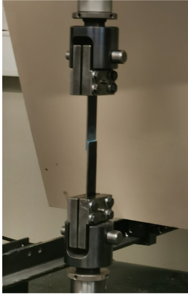
Figure 8: Single lap joint testing procedure.
