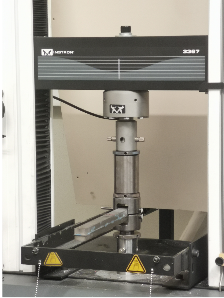
Figure 23: DCB testing procedure.
