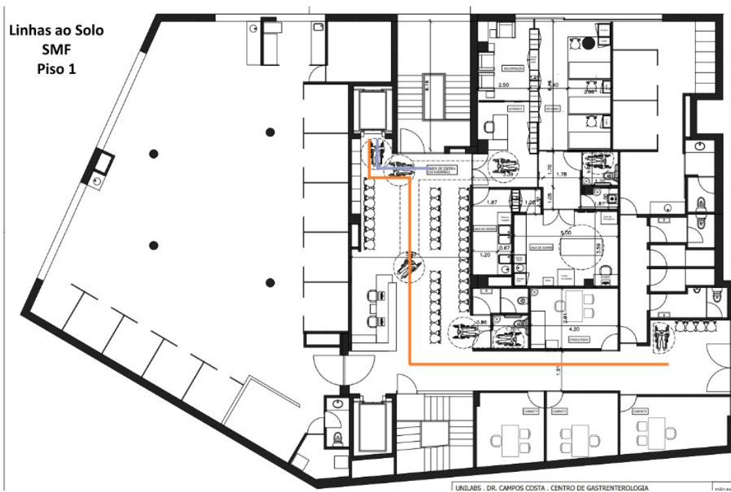
Figure 32: Ground lines planning of floor 1
