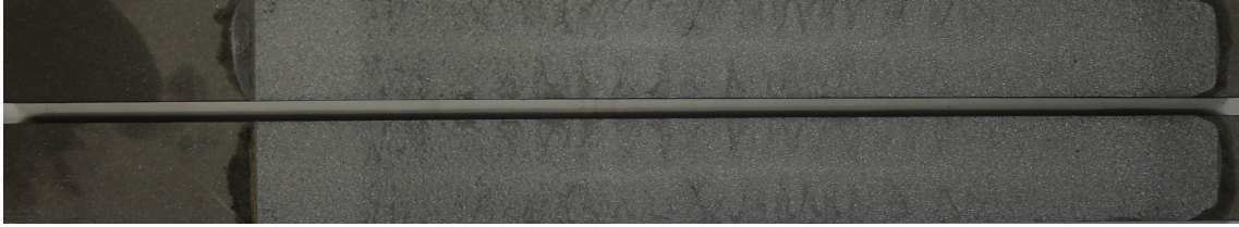
Figure 21: Representative fracture surface for ENF specimens in the neat state.
