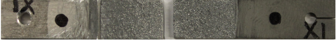
Figure 26: Representative fracture surface for SLJ specimens with 5% sphere content.
