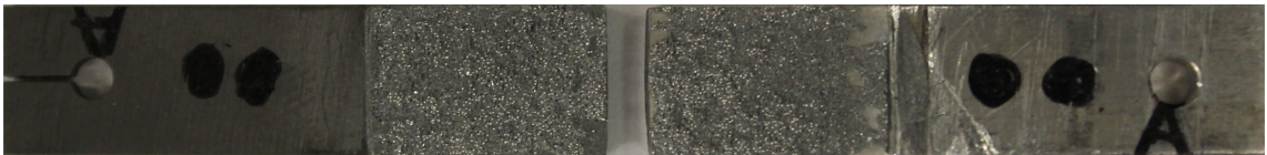
Figure 28: Representative fracture surface for SLJ specimens with 10% sphere content.
