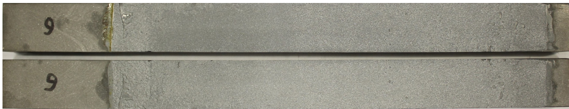
Figure 35: Representative fracture surface for ENF specimens with 5% sphere content.
