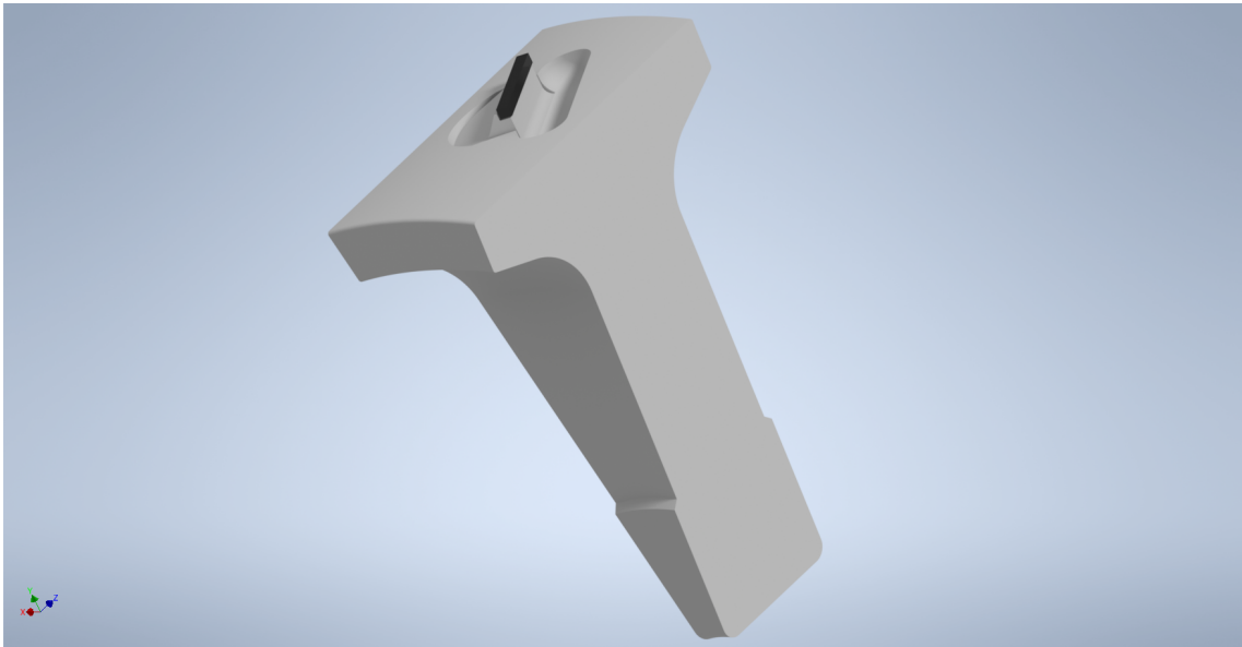
Figure 39: One bit partial edge milling tool 3D model obtained with Autodesk Inventor ® .
