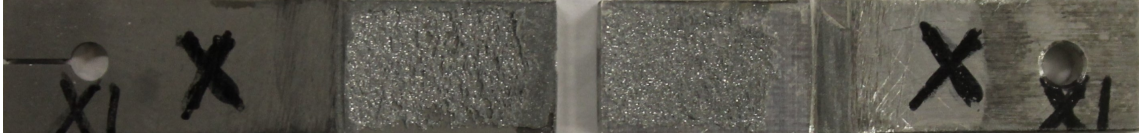
Figure 24: Representative fracture surface for SLJ specimens in the neat state.
