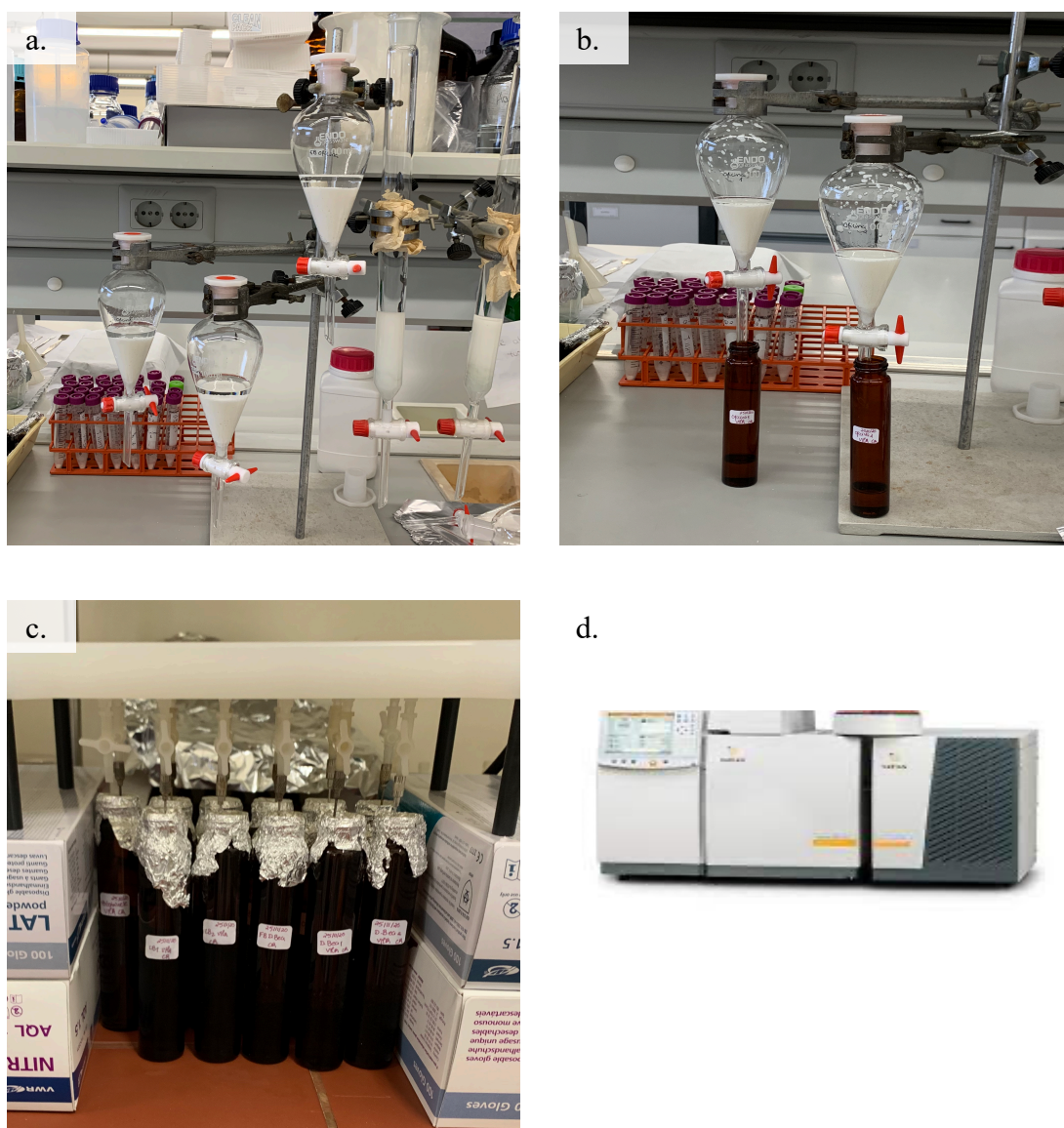
Figure 3. Main steps of the analytical protocol: Solid-liquid extraction (a and b), volume reduction through a stream of nitrogen (c), and quantification process (d).
