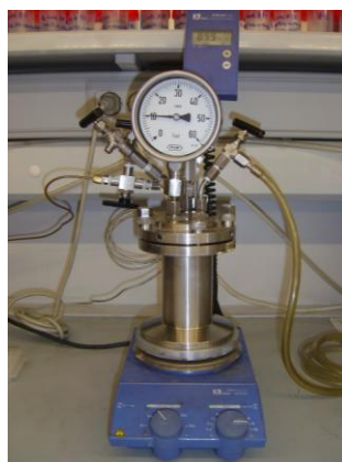
Figure 2.1 Schematic representation and photograph of the batch reactor used for the hydrogenation reactions.
