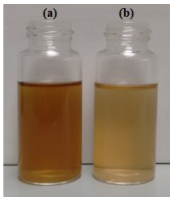
Figure 3.1 HISWL leachate samples: raw (a) and after treatment by catalytic oxidation H 2 O 2 and chemical precipitation as barite under stoichiometric conditions at the natural effluent pH (b).
