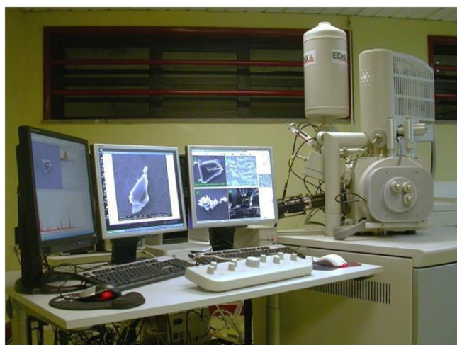
Fig. 2. 21: Illustration of the experimental setup used for SEM measurements.
