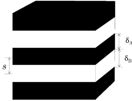
Figure 2.1 Striation thickness in an ideal lamellar structure.
