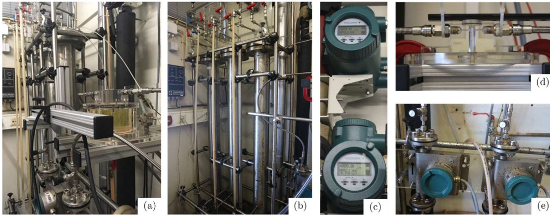
Figure 4.10 Photographs of CIJ experimental setup (a) full experimental setup; (b) pressurised tanks; (c) Coriolis flow meters screen; (d) CIJ mixer; (e) needle valves and Coriolis flow meter.
