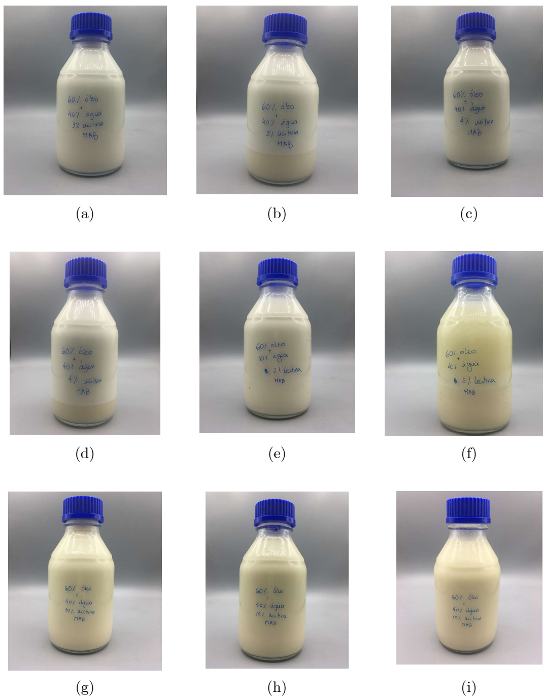
Figure 4.59 Stabilization analysis of o/w emulsions made with the rotor-stator mixer, for different mass fraction of lecithin (a) 1.3% on Day 0; (b) 1.3% on Day 1; (c) 1.7% on Day 0; (d) 1.7% on Day 1; (e) 2.1% on Day 0; (f) 2.1% on Day 1; (g) 4.1% on Day 0; (h) 4.1% on Day 1; (i) 4.1% on Day 6.
