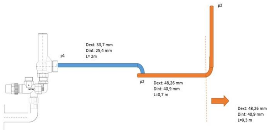
Figure 27 - PRV (52 bar) discharge piping and placement
