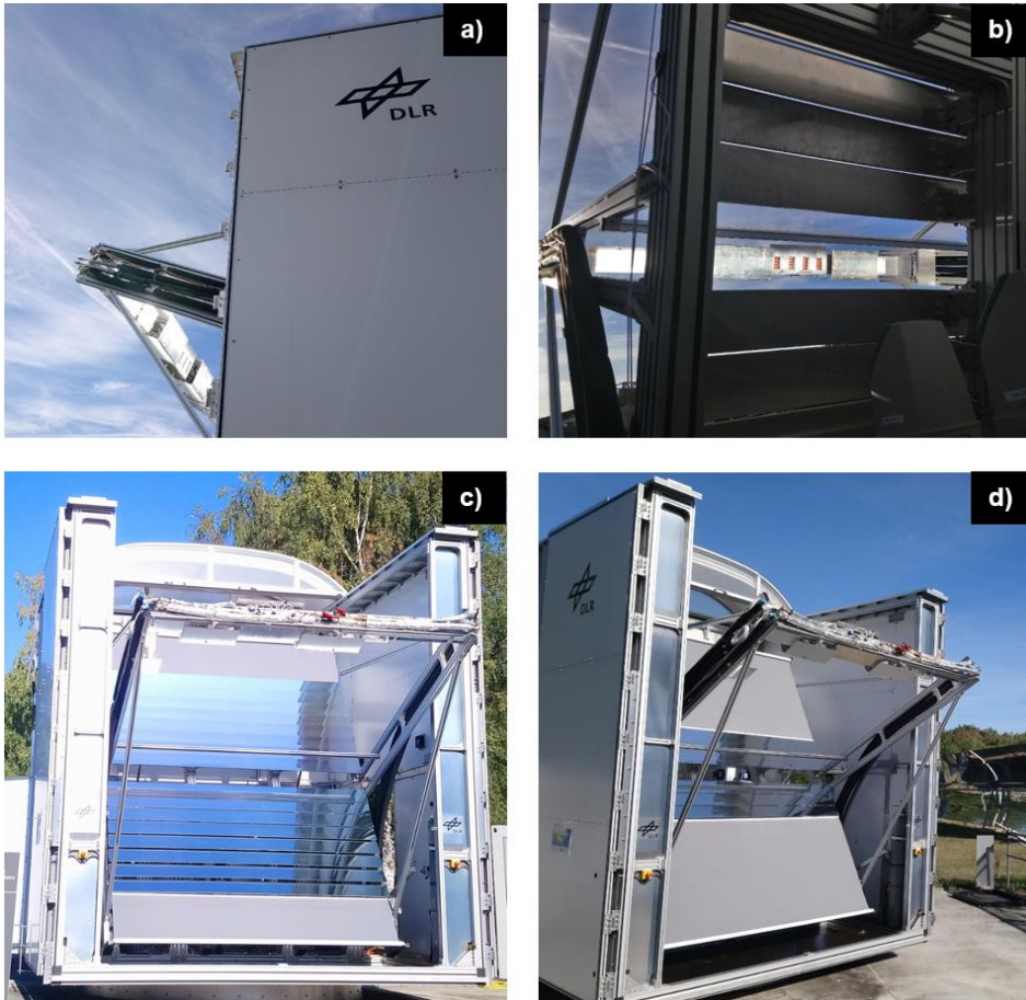
Appendix 5-f. CoolPEC module installed in the SoCRatus during operation under concentrated sunlight: a) front view of the module; b) view of the module from the back of the rectangular mirrors; c) SoCRatus being operated with 16 active mirrors; d) SoCRatus being operated with 6 active mirrors.
