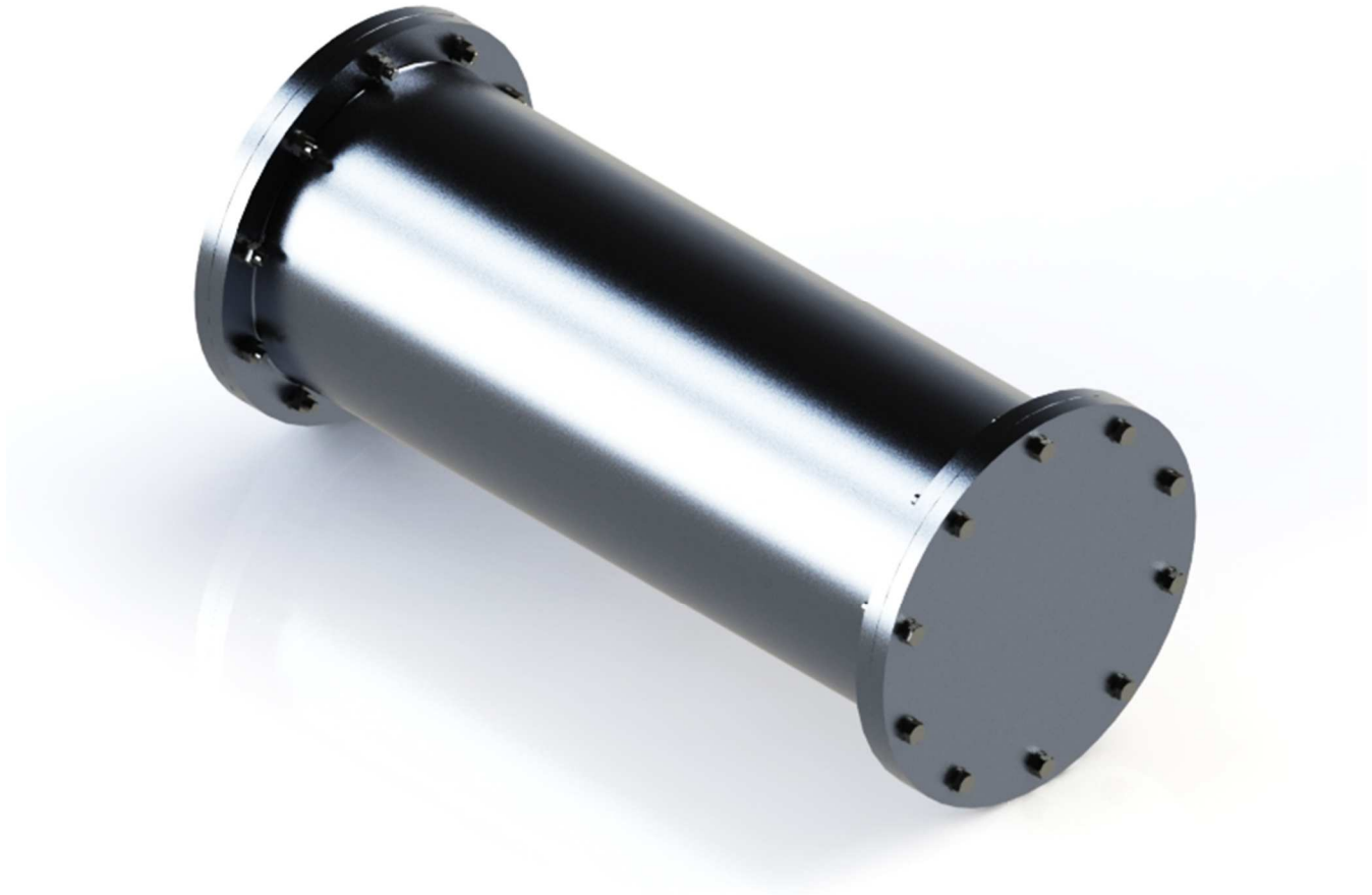
Figure 4.12. Rendered image of the SCC pressure vessel.
