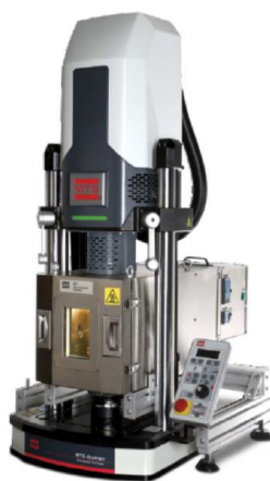
Figure 18 - Representation of the MTS Acumen™ 3 Test System equipment [37]
