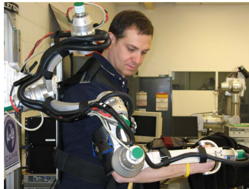
Figure 2.17: Exoskeleton Arm Developed by [16].
