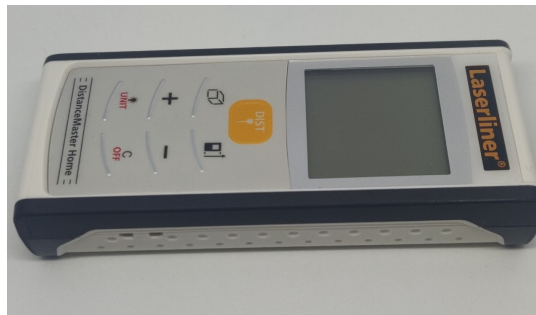
Figure 5.4: Laser used as a ground truth to measure the actual distance
