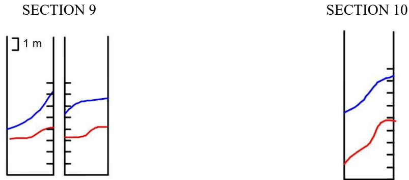
Fig. 80 - Graphic comparison of the free surface for sections 9 and 10 for the flow rate of 896 m 3 /s: Experimental results - blue line; GPUSPH results - red line.
