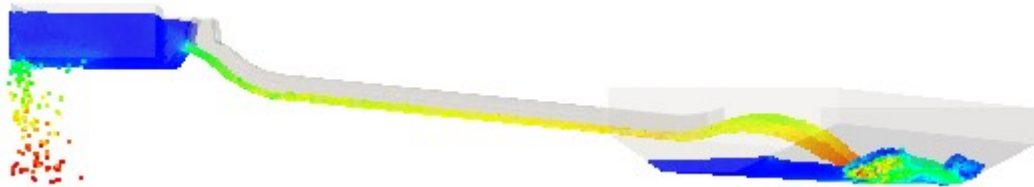
Fig. 100 – Illustration of a particle leakage problem in the upstream reservoir.
